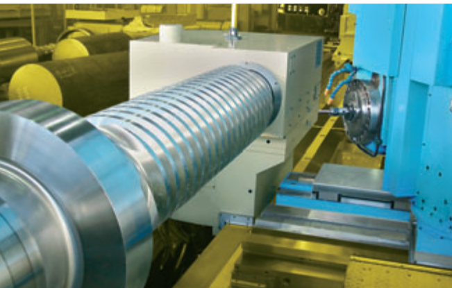
Milling of threaded spindle Ø 720 x 4,000 mm for screw press
