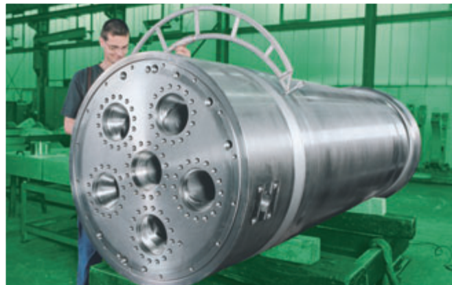
Press cylinder Ø 1,090 x 3,100 mm for the automobile industry
