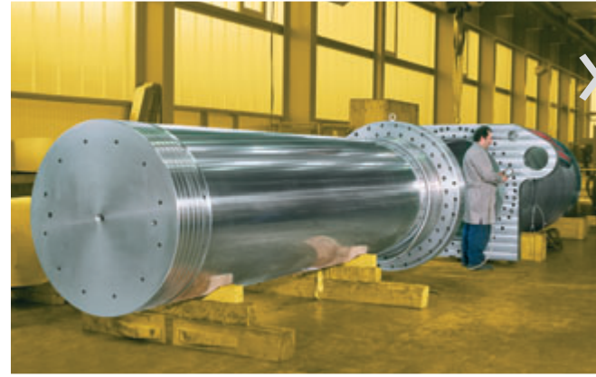
Hydrostatic cylinder for hydraulic pressure test for pipeline tubes, \varnothing 1,700 / \varnothing 1,260 \times 6,100 mm length, 52 tons
