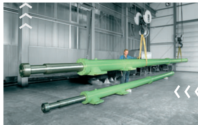
Feed cylinder (thruster) for manipulators in longitudinal forging press Ø 330 / Ø 190 x 11,500 resp. 16,200 mm length
