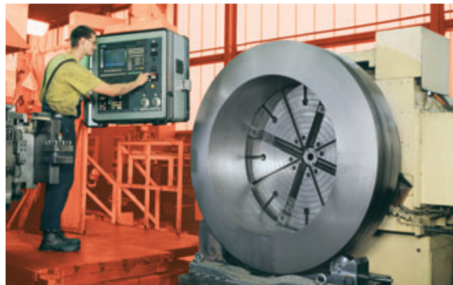
Spherical pressure ring Ø 1,875 x 510 mm for hydraulic cylinder—balancing of lateral force
