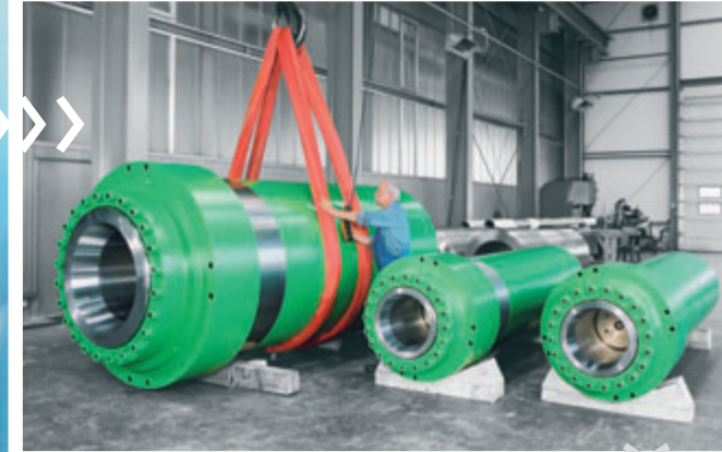
Main- and side cylinders for open-die forging press Ø 1,750 / Ø 1,070 x 3,500 mm length, 31 tons Ø 950 / Ø 545 x 3,250 mm length, 9 tons
