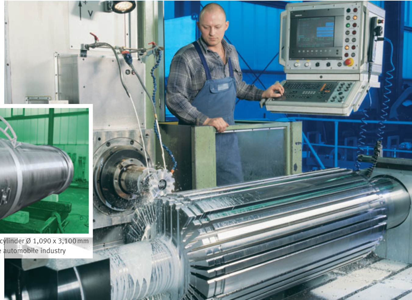
Generator shaft, milling of winding slots
