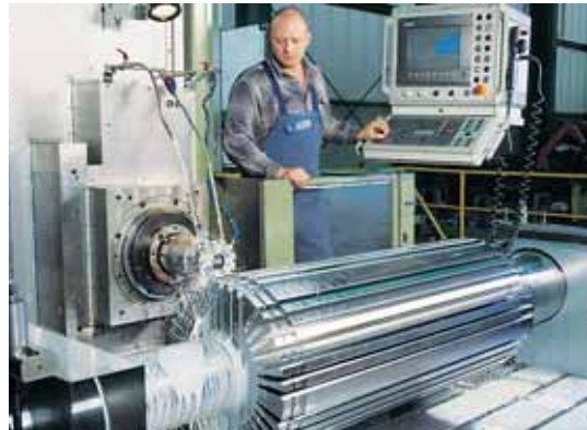
Generatorwelle, Fräsen von Wickelnuten Generator shaft, milling of winding slots
